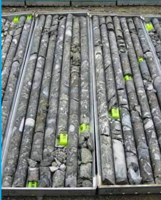
Kimberlite core from diamond drill borehole number DH12.
