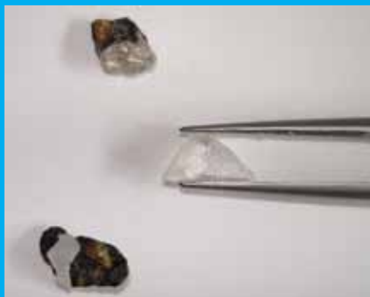
A high quality Type IIa Pure gem diamond in tweezers and in kimberlite host rock (bottom left).
